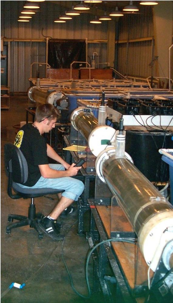
**Figure 44. Three swim respirometers used in this study being used at the NOAA NWFSC AquaLab.**
